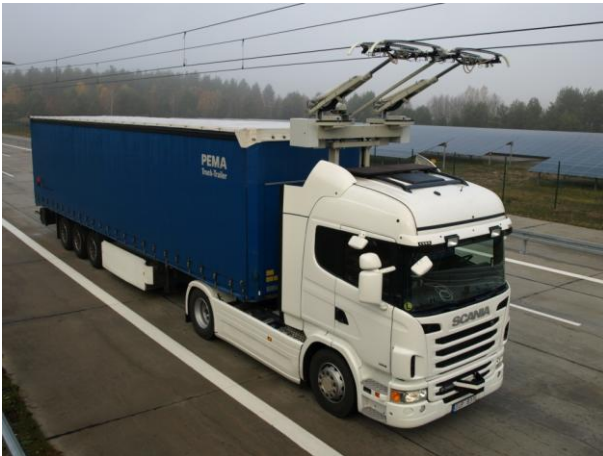
Conductive power transfer from overhead lines
