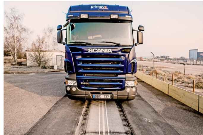
Inductive power transfer from the road
